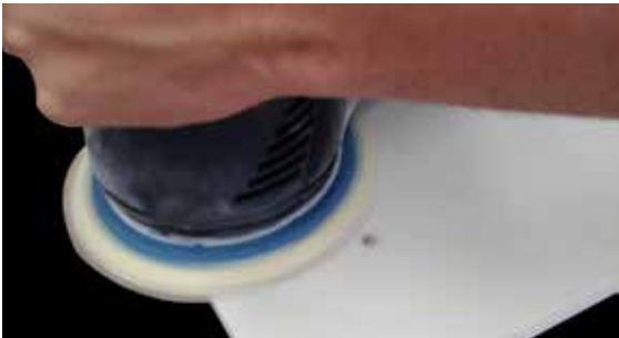
Remove the screw and sand away any surplus adhesive.
